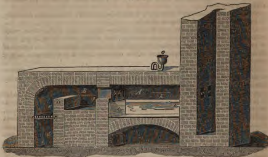
Furnace for converting Chloride of Sodium into Sulphate of Soda.
